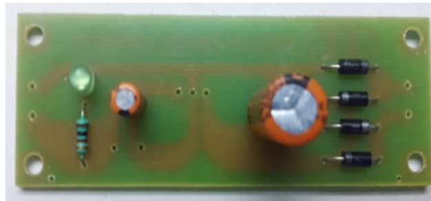
Fig 4.9 Power supply Assembled Board
