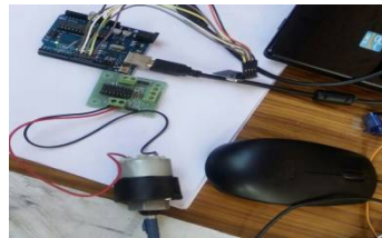
Fig3: shows how the motor works with motor driver
