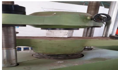
Fig 3.3 Testing of Compressive strength
