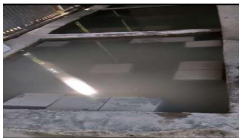
Figure 3.2 Curing of cube
