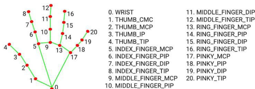
Fig 1.1 MediaPipe Structure for Hand Recognition
