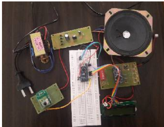
Figure 10. Prototype Output of Bus Alert System for Blind People
