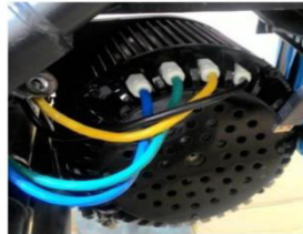
Fig 2: for 5kW BLDC 48V motor
