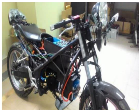
Fig 1: The retrofitted motorbike with the battery and BLDC motor
