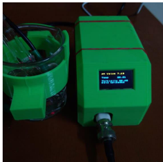
Fig. 6 The 3D Printed Product Casing Model
