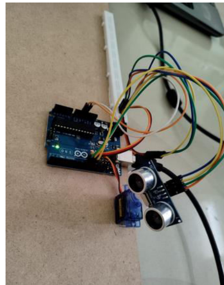
Fig 3: Model of RADAR with servo motor.
