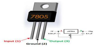
The input capacitor 0.33uF is a ceramic capacitor that deals with input inductance problems and the output capacitor 0.1uF is also a ceramic capacitor that adds to the stability of the circuit. These capacitors should be placed close to the terminals for them to work effectively. Also they should be of ceramic type, since ceramic capacitors are faster than electrolytic.
