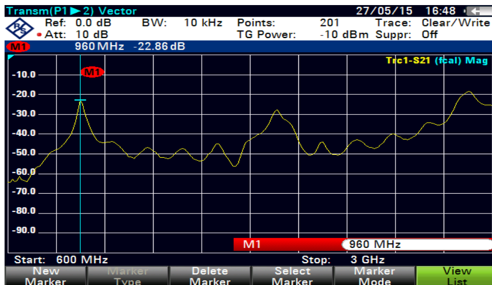
Figure 4: Measured S21 response
