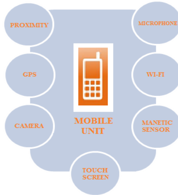
Fig. 1. Smartphone with embedded sensors
