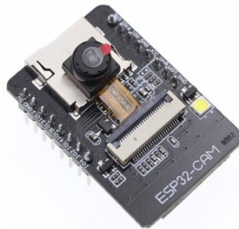
Fig 5: ESP32 Wi-Fi enabled camera
