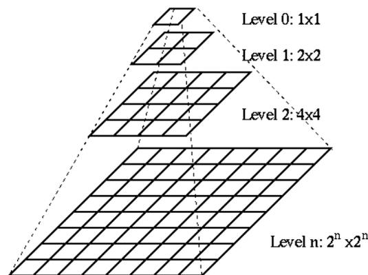
Figure 5: Laplacian pyramid structure
