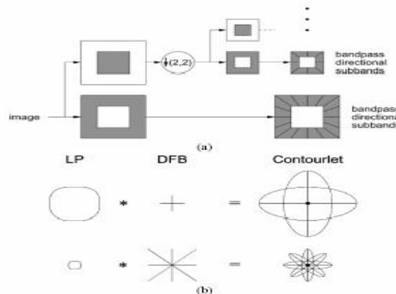
Figure 1.(a) Block diagram of a PDFB and (b) Supports for Contourlets
