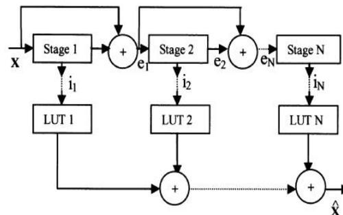
Figure 6. Multistage Vector Quantization Scheme
