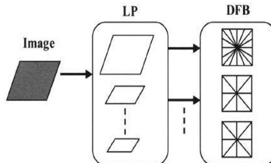
Figure 2. A flow graph of the Contourlet Transform
