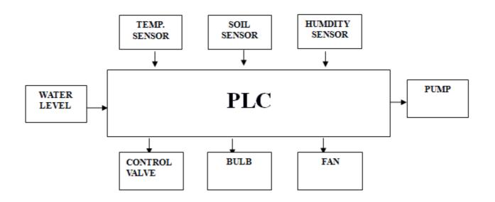
Different sensors are kept inside the mushroom plant which senses any variations in Parameters which are being monitored inside the plant and the sensors outputs are continuously compared with set point that of the standard conditions required for the mushroom plant. The output of the comparator is given to the PLC and the PLC switches on the corresponding actuators according to the program written in it. Thus the parameters required inside the mushroom plant are maintained automatically.
