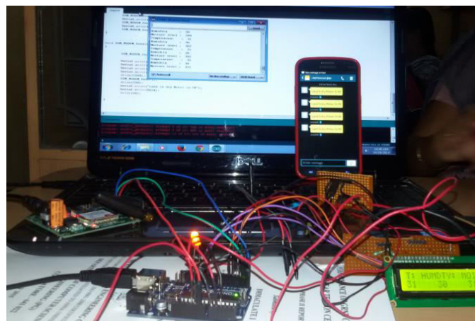
Fig. 11 GSM Interfaced with Arduino
