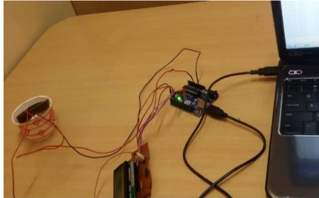
Fig. 9 Moisture Sensor is Interfaced in the Microcontroller
