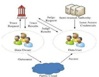
Authority is responsible for initializing system parameters and data user registration. Also, it handles the call request from the cloud in the first proposed construction.
