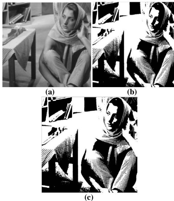
Figure 2: (a) Original Image, (b) Multi-thresholding, (c) Otsu's thresholding
