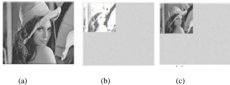
Fig. 2. (a) Original image Lena. (b) One level DWT in sub band LL (c) One level IWT in sub-band LL.
