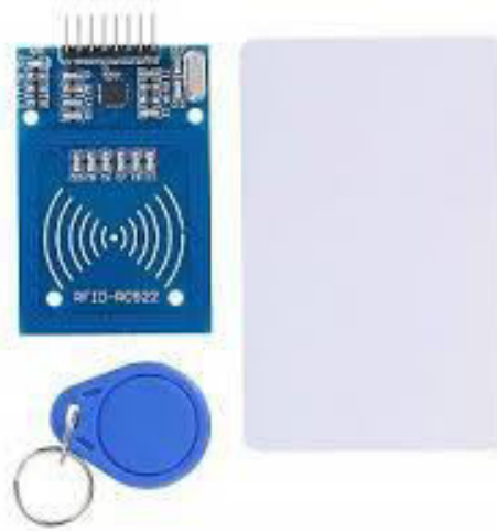
Figure 2: Image depicting MFRC522 RFID reader and RFID tag
