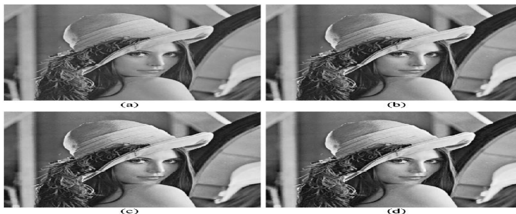
Fig. 4. The original and contrast-enhanced images of “Lena” by splitting 10, 15 and 20 pairs of histogram peaks in the proposed algorithm. (a) Original image of “Lena”. (b) 10 pairs: 0.185 bpp, 29.10 dB. (c) 15 pairs: 0.268 bpp, 25.97 dB. (d) 20 pairs: 0.345 bpp, 24.91 dB.
