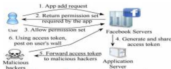
Fig.3. Steps involved in hackers using malicious applications to get access tokens to post malicious content on victims'
