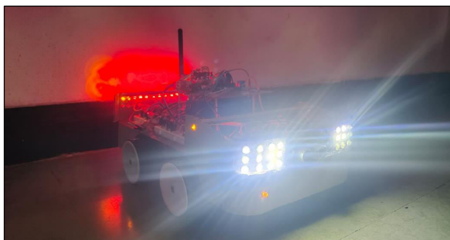
Fig No.10 Corner Lights On When Indicator Turns On
