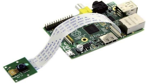
Fig.5: Connection of Camera module on Raspberry
