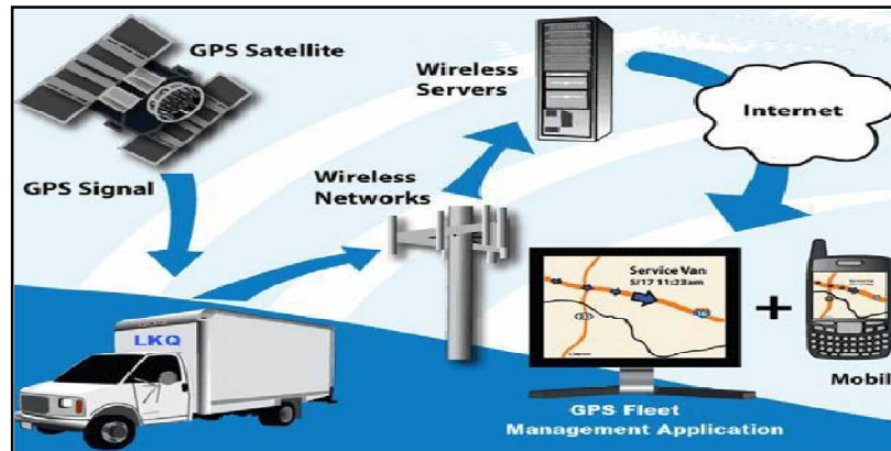
Fig 1. Object Tracking System Using GPS and GSM
