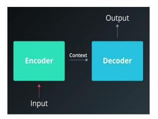
Since both the encoder and decoder are recurrent, they have loops which process each part of the sequence at different time steps. To picture this, it's best to unroll the network so we can see what's happening at each time step.
