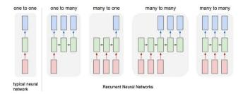
Each rectangle is a vector and arrows represent functions (e.g. matrix multiply). Input vectors are in red, output vectors are in blue and green vectors hold the RNN's state (more on this soon).
