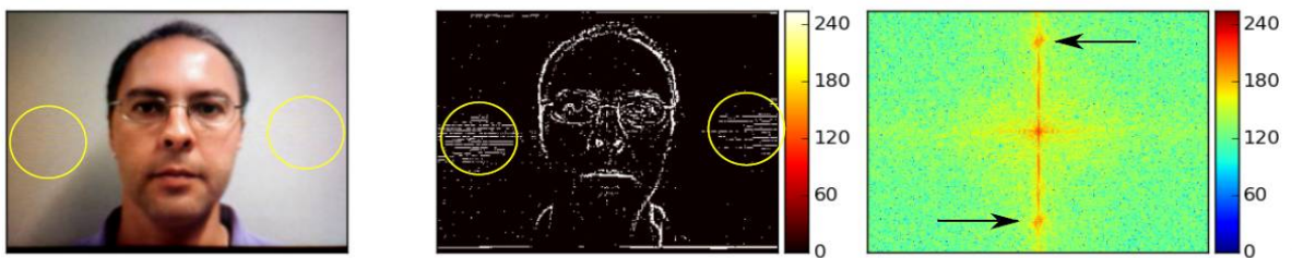
b. Mobile attack video, its residual noise video, and corresponding magnitude spectrum.
