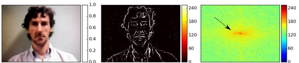
c. Another mobile attack video, its residual noise video, and corresponding magnitude spectrum.
