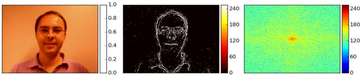
a. Valid access video, its residual noise video, and corresponding magnitude spectrum.
