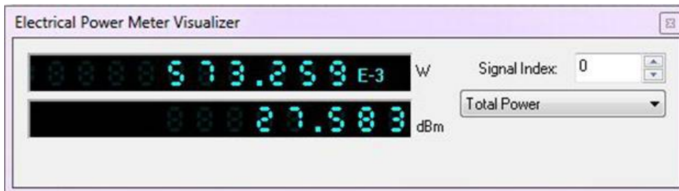
Figure 8. Electrical power output of CATV system with external modulation.
