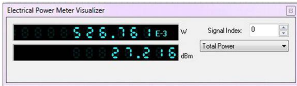
Figure 7. Electrical power output of CATV system with direct modulation.
