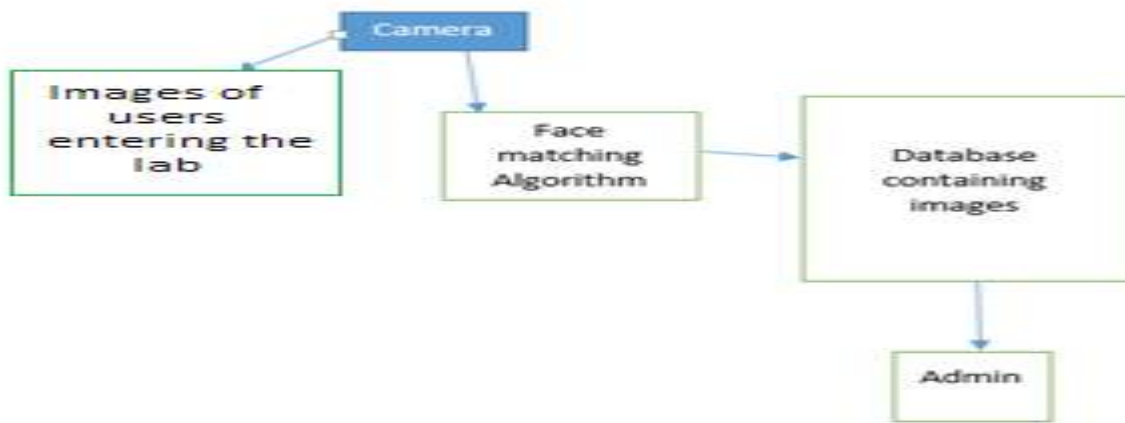
Fig-1: Basic working of face recognition system
