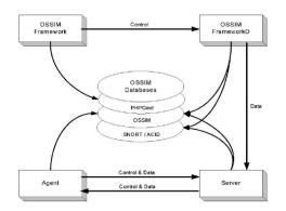
Figure.2 Functional Interaction among different Components of OSSIM
