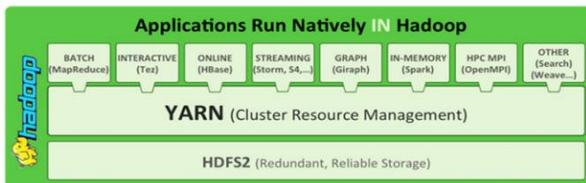
Figure 1 : Hadoop Ecosystem using YARN Cluster Resource Management and Depicting the Applications Run Natively in Hadoop over the HDFS (Hadoop Distributed File System)
