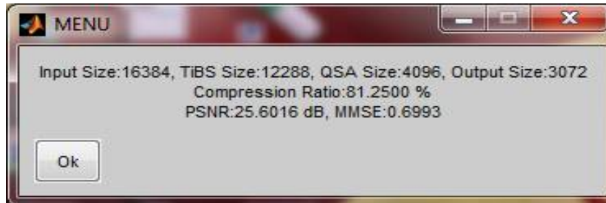
Fig.9.Theoretical result of Compressed and Decompressed Image by using QSA and TiBS Algorithm
