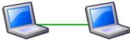
Fig. 1.2 Peer-to-Peer or ad-hoc wireless LAN
