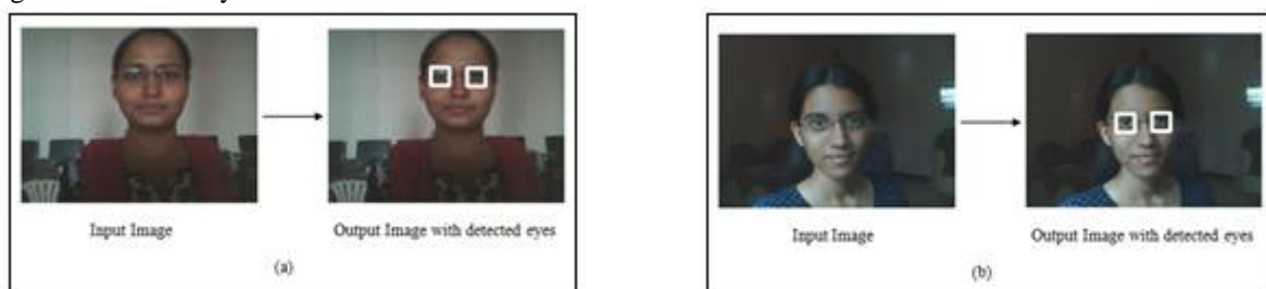
Fig.7. Detection of eyes through spectacle from input images captured by Dell Laptop's integrated web camera with 1.0 Mega Pixel. (a) and (b) Images containing single person wearing spectacle as an input and its detected eyes images as output.
