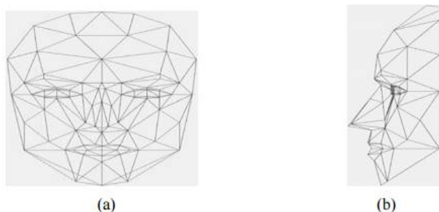
Fig 4: The CANDIDE model in frontal and profile view
