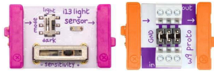
Fig 5. Receiver components: Light sensor and proto bits
