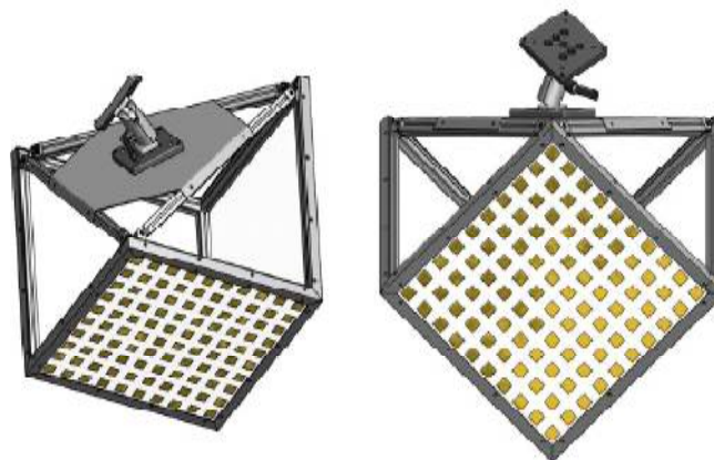
Fig 4: Massive MIMO antenna
