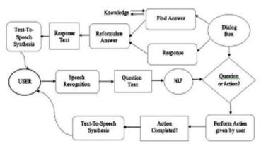
The above fig. shows the workflow of the basic process of voice assistant. Speech recognition is used to convert the speech input to text. This text is then fed to the central processor which determines the nature of the command and calls the relevant script for execution.
