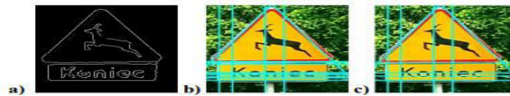
Fig. 3.5. Line detection: a) sample image used for line detection b) detected lines for given parameters of Hough transform c) Reduced set of lines detected in the image.
