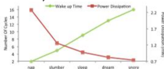
Fig. 5. Tradeoff between wake-up time and power consumption with five power-off modes.
