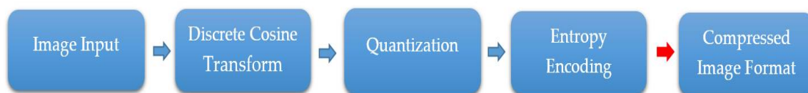
Figure 2: Block Diagram of JPEG Image Compression
