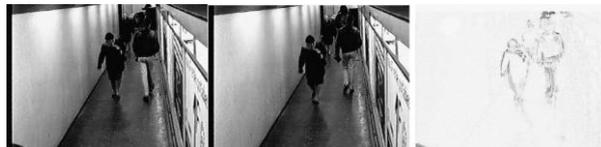
Fig.1.Example of temporal difference technique used in motion detection.
