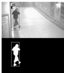
Fig. 2. Example of background subtraction technique used in motion detection.
