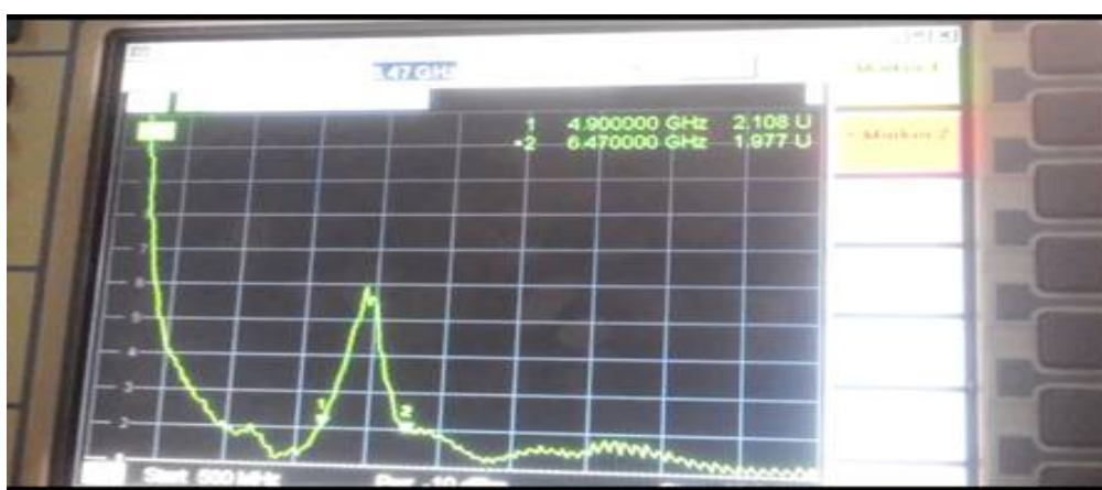
Fig.10. VSWR Measured on Network Analyzer
