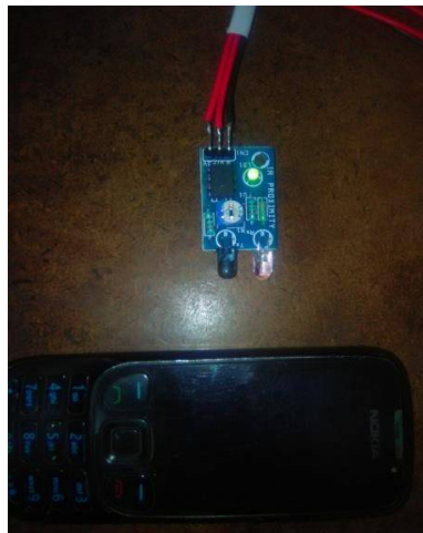
Fig 5.7 shows the Infrared Sensor output in presence of object before the sensor transmitter and receiver in which the LED blinks when the sensor which detects the presence of obstacles in the moving path.
