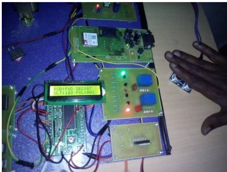
Fig 4.2 shows ultrasonic output when it reaches the maximum level of the sensor.
