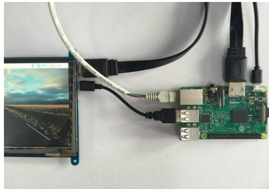
Figure 1. Hardware Architecture of Smart Mirror
