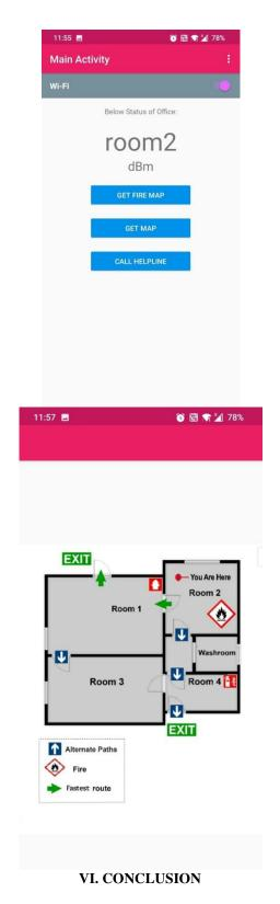
The users equipped with mobile phones or PDAs interact with the sensors through Wi-Fi.GPS is inadequate for indoor location positioning. Wi-Fi is a technique used for location tracking with wireless access points (AP's). Base on the range of wifi we can predict the current location of user in the indoor. Based on the current location we can show the
