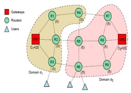
Fig 4: Mesh network divided into domains for load balancing [8]
