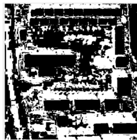
Fig. 7. Binary shadow map. Shadow effect is in white area while non-shadow is in black area.
