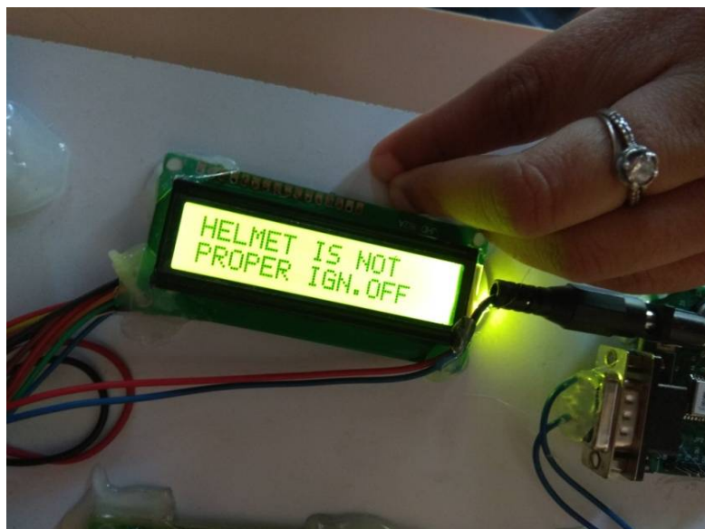
Fig.6: The bike won't start till the rider puts on the helmet. So, it will remind the rider by displaying the message "Helmet is not proper ignition off".
