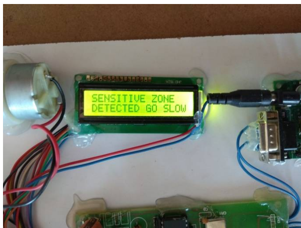
Fig.9: When bike enters sensitive areas it will display “Sensitive zone detected-Go slow” on LCD.
