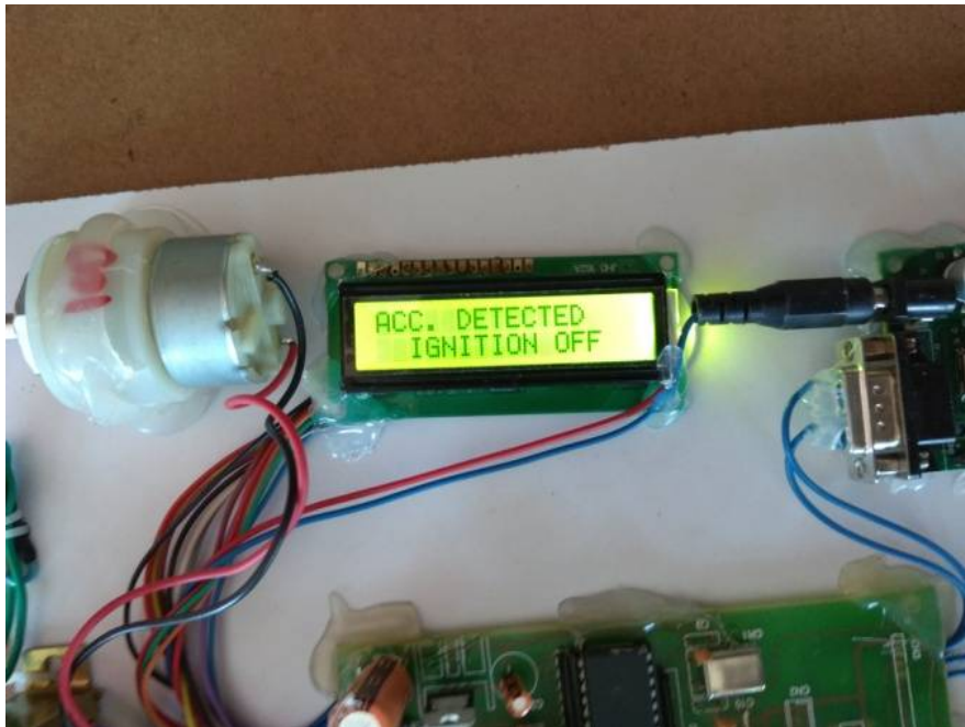
Fig.8 (a): When the accident occurs it will display that “Acc. Occurred Ignition off” and the sends the message to selected numbers.
