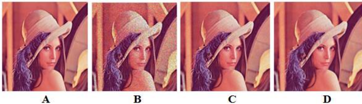
Fig.3: A. origin image. B. noisy image with speckle noise. C. image after de-noising using SVD. D. image after de-noising using SVD+TLS.
