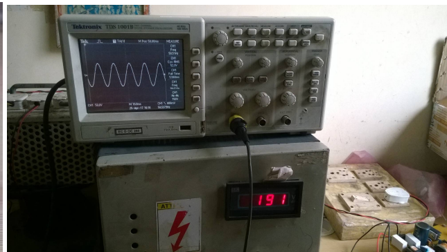
Figure 8: experimental result of prototype for 200 input dc and 115 output ac
