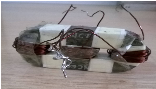
Figure 7: 3-phase inductor with umnccc-7 core
