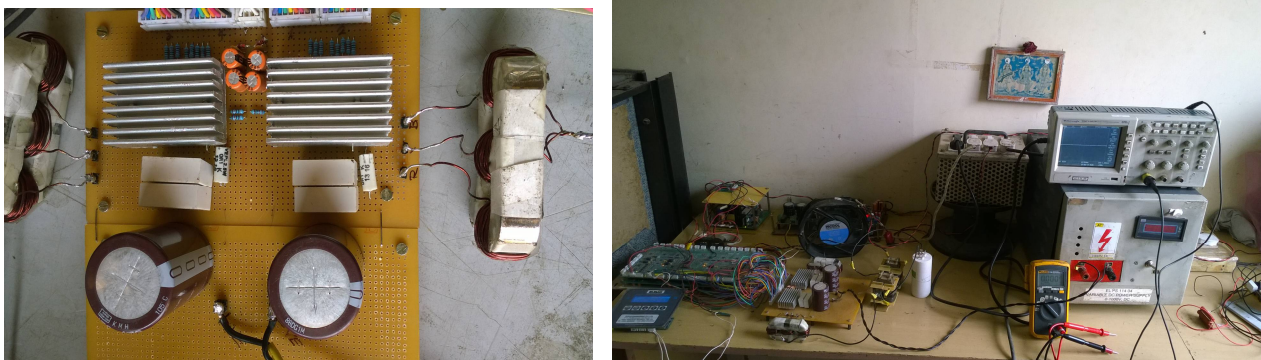
Figure 6: Hardware set up for single-phase 7-level inverter
